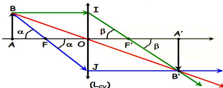
$$\alpha = \frac{\overline{AB}}{-\overline{FA}} = \frac{\overline{JO}}{-\overline{OF}} \quad ; \quad \beta = \frac{-\overline{A'B'}}{-\overline{F'A'}} = \frac{\overline{OI}}{\overline{OF'}}$$
